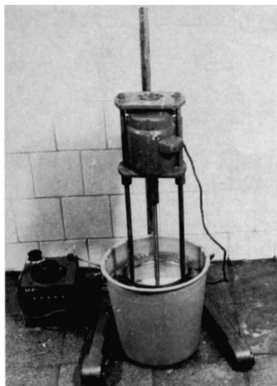
Figure 1—Setup for microcrystallization.
